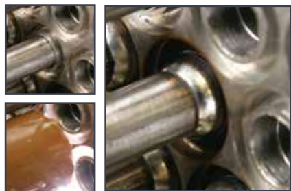
Orbital welding of element to tubesheet
